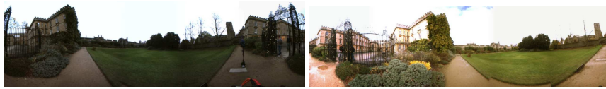
Fig. 3 Example place recognition result generated by FABMAP under markedly different lighting conditions. Probability of loop closure is calculated to be 0.9519.
