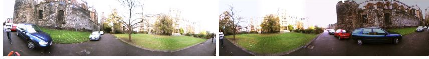
Fig. 2 Place recognition results generated by FABMAP. Probability of loop closure is calculated to be 0.9986. (Note that a stitched panorama view is shown here; the algorithm is applied directly to the unstitched frames.)
