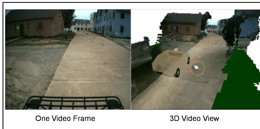
Fig. 1 3D Video View of a Mobile Robot. Left: A video frame produced from a camera on a moving vehicle. Right: The 3D Video view produced from all of the video that has been received in the last few seconds by the vehicle. The operator can look at this database from any angle, at any zoom, while it continues to be updated in real time. The vehicle is synthetic since no sensor has imaged it, but the rest of the content is generated from live video produced by the forward looking sensor mounted on the vehicle roof.
