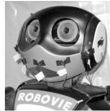
Fig. 3 SIG2 has 8 microphones on its body.
