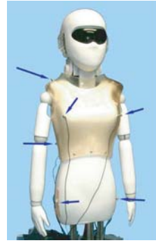
Fig. 3 SIG2 has 8 microphones on its body.
